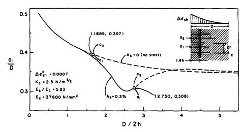
Fig. 5. Relative length of shrinkage or cooling cracks for reinforcement deeper within the solid.
