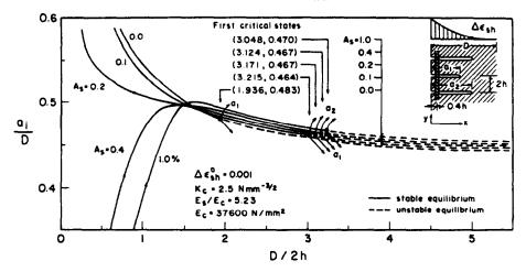
Fig. 4. Relative length of shrinkage or cooling cracks for reinforcement close to surface.
