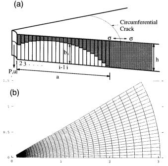
FIG. 2. Diagram of: (a) Subdivision into Vertical Crack Strips for Purpose of Numerical Analysis; (b) Mesh Used for Calculating Compliance Functions of Plate Wedge
