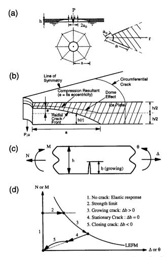
FIG. 1. Diagram of: (a) Vertical Cross Section of Floating Sea Ice Plate, Crack Pattern Viewed from Top and Plate Wedge between Two Adjacent Radial Cracks; (b) Half of Plate Wedge with Part-Through Crack Profile and Schematic Representation of Compression Resultant Elevation Showing Dome Effect; (c) Bending Moment and Normal Force Acting on Cracked Cross Section, and Additional Rotation and Displacement due to Crack; (d) Stages in Evolution of Vertical Crack Strips
