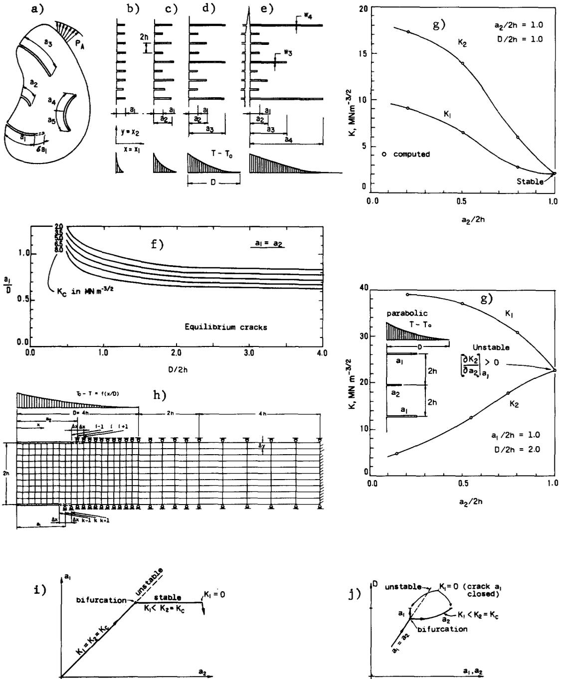
FIG. 1 General and Special Crack Systems Investigated (a-e), Some Numerical Results (f,g) with Grid Used (h;  $2h = 1\text{m}$ ), and Bifurcation of Equilibrium Path (i,j)
