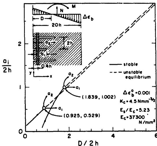
Fig. 7. Critical states and growth of bending cracks.
