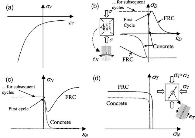
**Fig. 5.** Boundary surfaces for kinematically constrained model: (a) volumetric boundary; (b) fiber resistance mechanism in uniaxial compression (left) and deviatoric boundary (right); (c) normal boundary; (d) shear boundary (left) and fiber resistance mechanism in triaxial compression (right)
