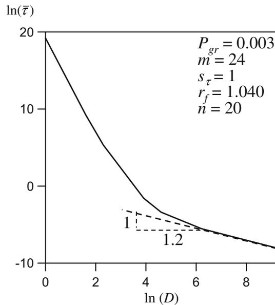
Fig. 4. Size effect on mean structural lifetime.
