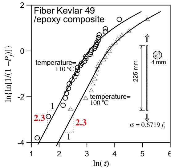
Fig. 3. Optimum fits of experimental lifetime histograms Kevlar 49 fiber composites tested at temperatures of 100 °C and 110 °C.
