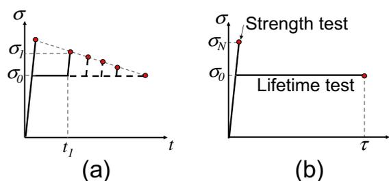
Fig. 1. (a) General loading history (b) loading histories for strength and lifetime tests.
