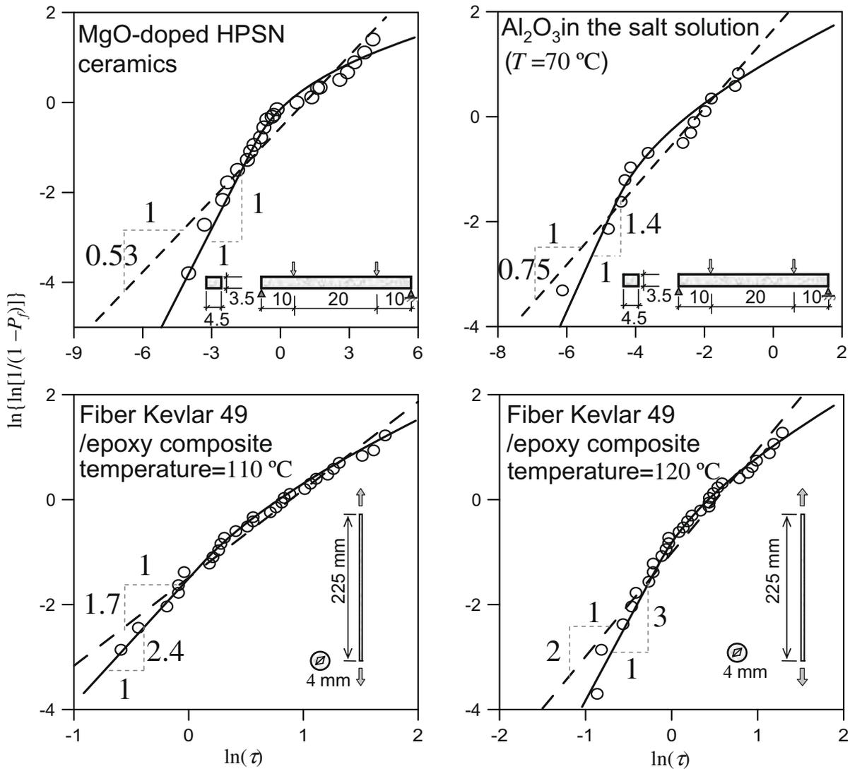
**Fig. 2.** Optimum fits of experimental lifetime histograms of ceramics and Kevlar 49 fiber composites by the present theory and the two-parameter Weibull distribution: (a) MgO-doped HPSN ceramics, (b) Al<sub>2</sub>O<sub>3</sub> in the salt solution, (c) Fiber Kevlar 49/epoxy composite at 110 °C and (d) Fiber Kevlar 49/epoxy composite at 120 °C.
