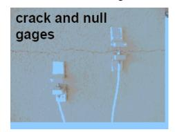
Figure 0: Photograph of Micro-meter Crack Displacement Sensors
