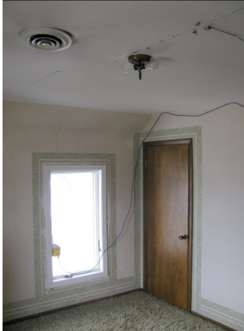
← b - Interior view of Node 3 in upstairs bedroom. Crack sensor connected to eKo Mote
