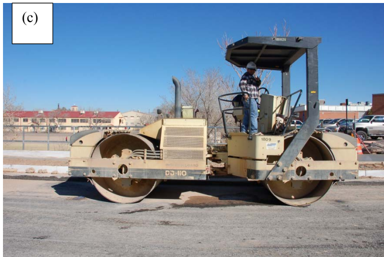
Figure III-7 - Road during compaction process (a) and equipment used: Dynapac CA260 (b), Ingersoll-Rand DD10 (c), CAT CB534D (d)
