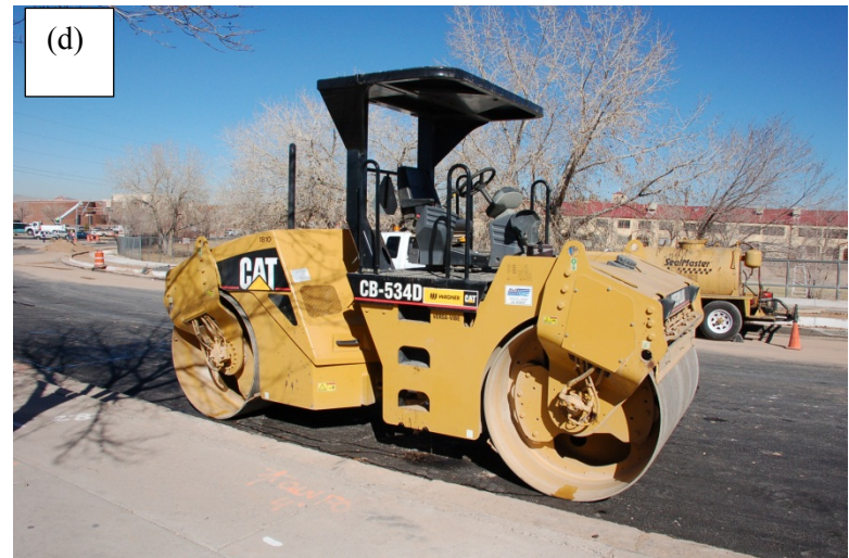
Figure III-7 - Road during compaction process (a) and equipment used: Dynapac CA260 (b), Ingersoll-Rand DD10 (c), CAT CB534D (d)
