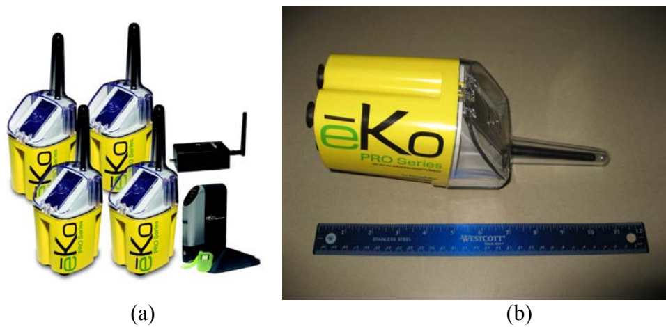
Figure B-3: (a) eKoPro Series WSN including base station, after Crossbow Technology, Inc. (2009a) (b) Individual eKomote with a 12-inch ruler for scale
