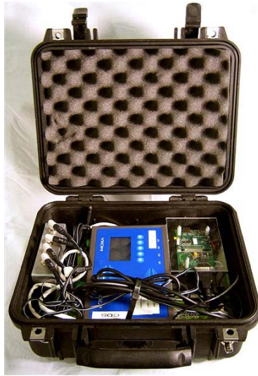
Figure A-6: Photograph of the base station of Version 3 of the wireless ACM system, including UC-7420, MIB510CA, cellular router, power distributor, and industrially-rated housing
