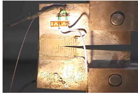
Figure B-13: Test coupons with crack propagated through (a) narrow gauge and (b) wide gauge affixed with elevated-temperature-cured adhesive
