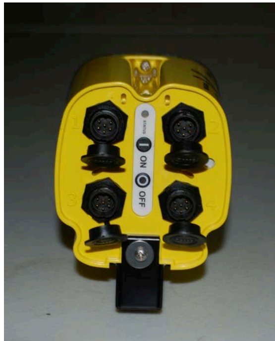
Figure E-7. Wireless node weatherproof enclosure and access ports.
