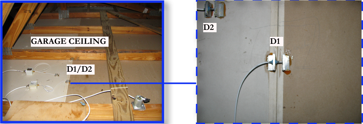
Figure X - Left: Instrumentation on uncracked drywall joint in garage ceiling Right: Close-up of gauges to measure in-plane response of joint and panel
