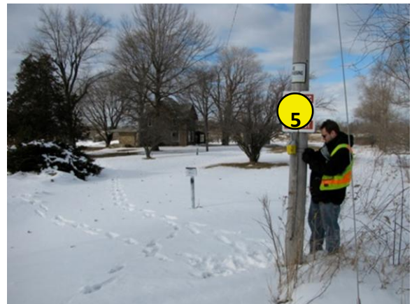
Figure 2.5 - Node 5 as relay point on telephone pole
