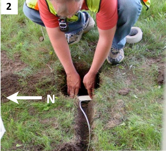
Figure 2.17 - 1 - Southeast corner of house showing seismograph (triaxial geophone) location 2 - View from house of trench and buried geophone 3 - Close-up of buried geophone with longitudinal axis pointing north toward the quarry
