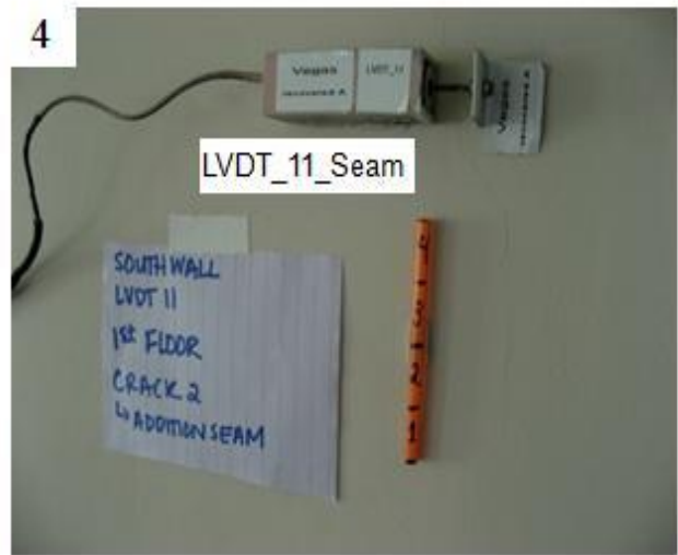
Figure 2.19 - 1 - Overall view of sensor suite on south wall (first floor) 2 - Closer view of suite on south wall 3 - Close-up of Shear crack monitored by LVDT_9 and Null gauge LVDT_10 4 - Close-up of Addition Seam crack monitored by LVDT_11 5 - Close-up of midwall geophone monitored by HG_16
