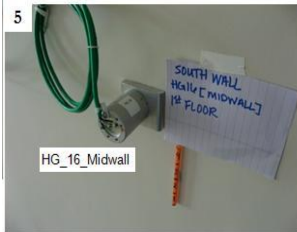
Figure 2.19 - 1 - Overall view of sensor suite on south wall (first floor) 2 - Closer view of suite on south wall 3 - Close-up of Shear crack monitored by LVDT_9 and Null gauge LVDT_10 4 - Close-up of Addition Seam crack monitored by LVDT_11 5 - Close-up of midwall geophone monitored by HG_16
