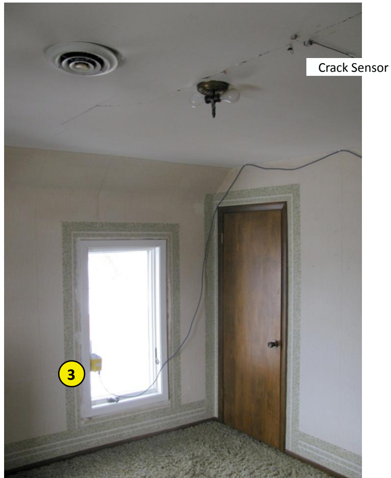
Figure 2.10 - Interior view of Node 3 in upstairs bedroom. Crack sensor connected to eKo Mote.
