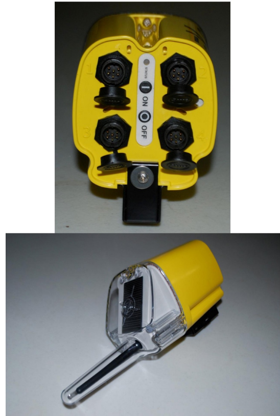
Figure 7 Wireless node weatherproof enclosure and access ports.
