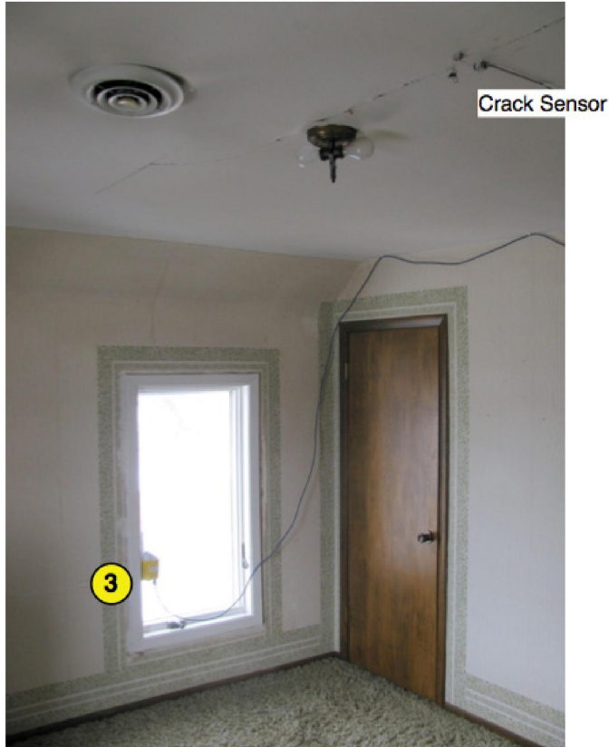
Figure 6: Context of node 3 and ceiling crack sensor. A close-up photograph of the ceiling crack and potentiometric proximity sensor is shown in Figure 8.
