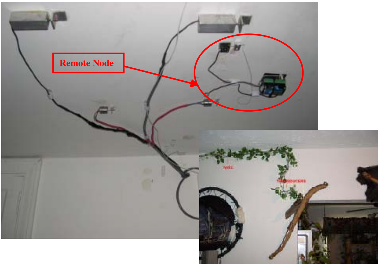
Figure 2.6: Plastic Ivy used to hide wires and sensor (bottom right) and the wireless remote node on the ceiling
