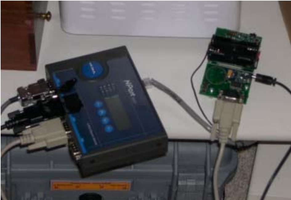
Figure 2.4: MOXA NPort (left) and MIB510 with mote running TOSBase (right)
