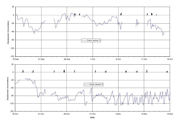
Figure 9: Comparison of Long-Term and Vibratory Response of Crack 3
