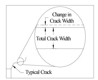
Figure 2 Definition of the change in crack width hearafter called crack displacement.
