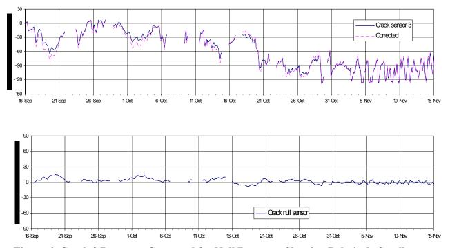
Figure 6: Crack 3 Response Corrected for Null Response Showing Relatively Small Effect of the Null Response
