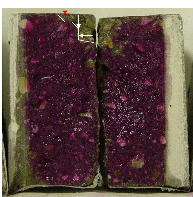
Figure 3.23. Round 2 sample showing outward curve carbonation front. White arrows indicate the direction of gas penetration and the subsequent carbonation front progression. Red arrow identifies carbonation ‘tail’ as described above.
