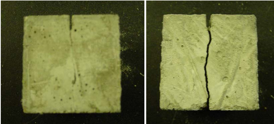
Figure 3.6. Side view of round 1 samples with saw-cut notch before and after cracking with a chisel and hammer.
