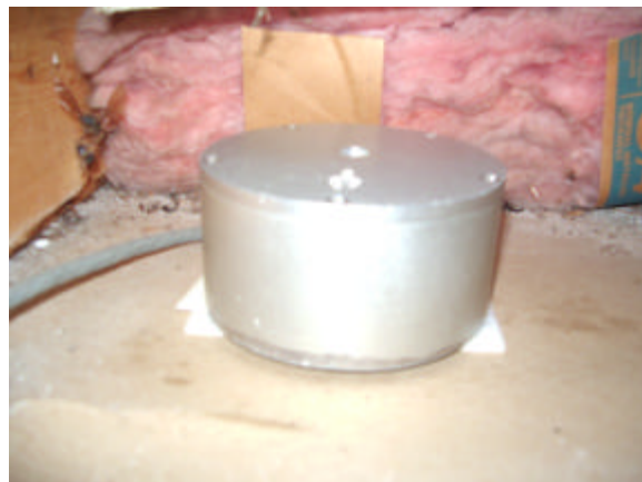
Figure 2.29 Picture showing the placement of the velocity transducer near the attic rafters
