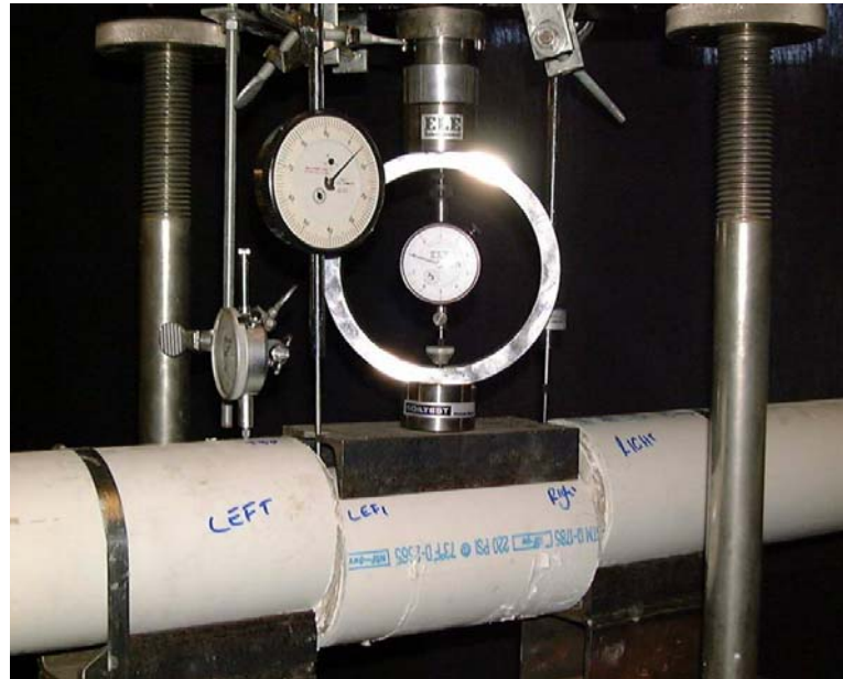
Figure 6. Apparatus for shearing cable-grout composites.
