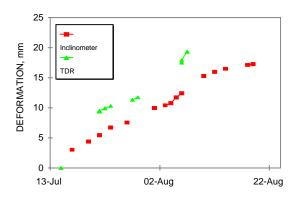
Figure 4-Comparison of TDR and inclinometer deformation time histories.
