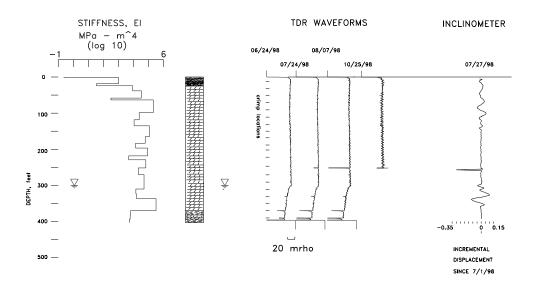
Figure 3-TDR waveforms and inclinometer profile indicating rock deformation beneath road adjacent to quarry.
