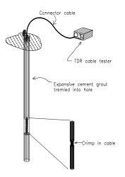
Figure 1-Schematic of cable installation and monitoring.
