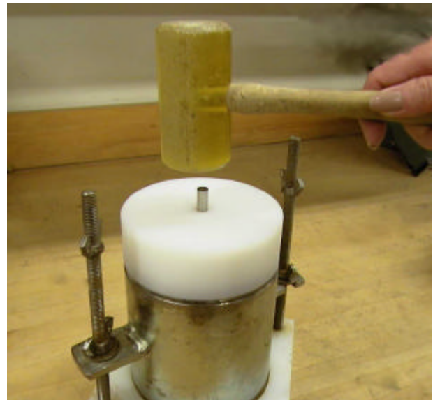
Fig. 1. Center Rod Being Driven into Specimen Through Guide Template
