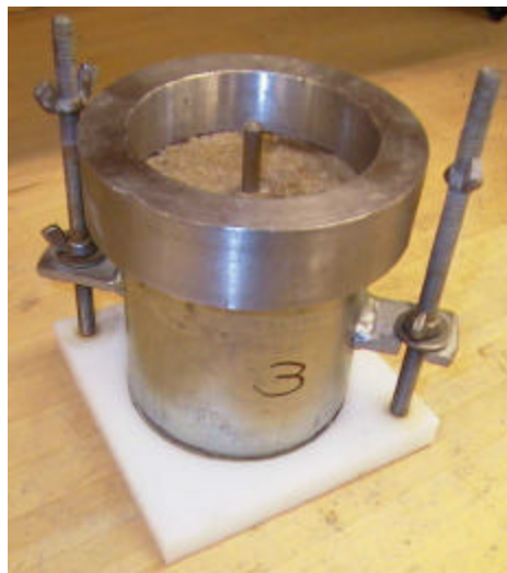
Fig. 2. Mold with Center Rod and Adapter Ring Ready for Multiple Rod Probe Head
