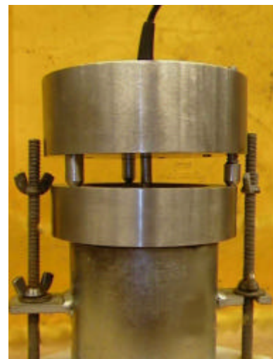
Fig. 1. Center Rod Being Driven into Specimen Through Guide Template
