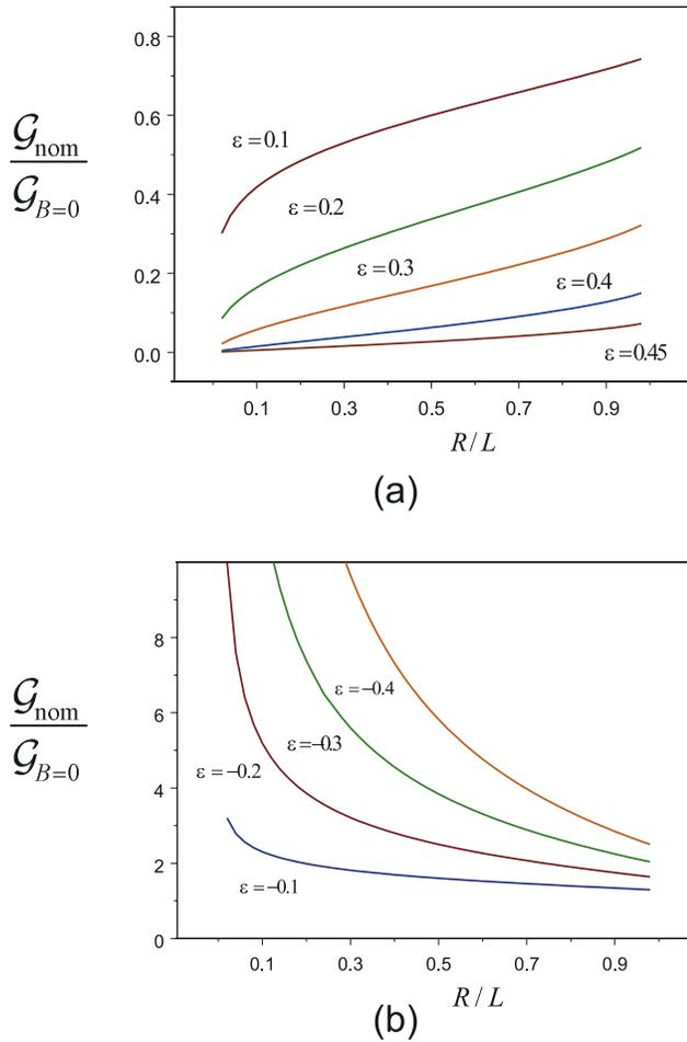
**Figure 9.** Nominal energy supplied by the applied loads  $\mathcal{G}_{\text{nom}}$  divided by the material value in the absence of porous media effects  $\mathcal{G}_{B=0}$  against  $R/L$  for (a) five positive values of the velocity-dependent parameter  $\varepsilon = 0.1, 0.2, 0.3, 0.4$  and  $0.45$  and (b) four negative values  $-0.1, -0.2, -0.3,$  and  $-0.4$ .
