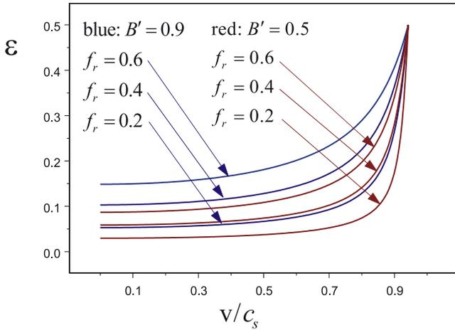
**Figure 4.** Variation of  $\varepsilon$  with  $v/c_s$  for undrained Poisson's ratio  $\nu_u = 0.4$ , three values of the friction coefficient and two values of the effective Skempton's coefficient  $B'$ .
