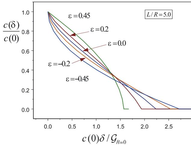
**Figure 10.** Relation for the cohesive part of the stress drop  $c(\delta)$ , divided by  $c(0) = \tau_p - \tau_r$ , versus relative slip, multiplied by  $c(0)/\mathcal{G}_{B=0}$ , implied by the solution. Shown for  $L/R = 5.0$  and several values of  $\varepsilon$ .
