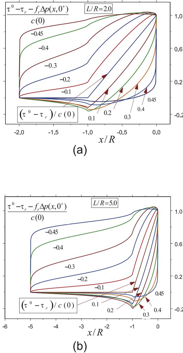
**Figure 7.** Effective frictional resistance minus  $\tau_r$  (divided by  $c(0) = \tau_p - \tau_r$ ) for (a)  $L/R = 2.0$  and (b)  $L/R = 5.0$ . Curves are labeled by positive and negative values of  $\varepsilon$ . Also shown is the nominal slip weakening in the absence of pore pressure changes  $\tau^0$ .
