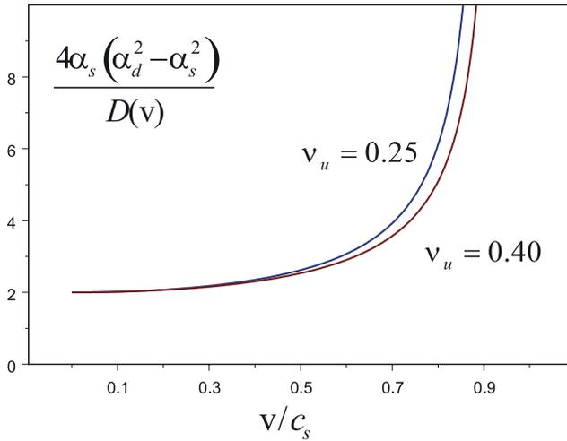
**Figure 3.** Velocity-dependent portion of  $k$  (first bracket in (13)) against the rupture velocity  $v$  divided by the shear wave speed  $c_s$  for two values of the undrained Poisson's ratio, 0.25 and 0.40.
