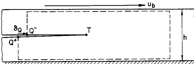
Figure 5 Idealization of a long strike-slip fault loaded by displacements u_b . Relative slip at point Q is \delta_Q .
